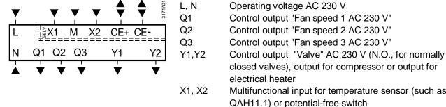
Multifunctional input for temperature sensor (such as
