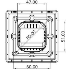
ARG800.1 single mounting frame for RDF800KN/NF
