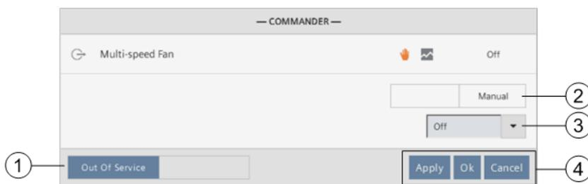
Figure 4: Commander dialog box for a Binary Object.
