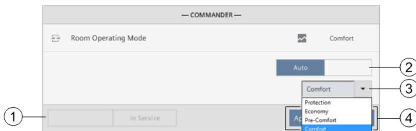
Figure 5: Commander dialog box for a Multistate Object.
